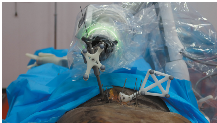
FIGURE 5 The surgeon used the trephine to remove a part of the lamina with the R-Pharos miniature parallel surgical robot assistance.
