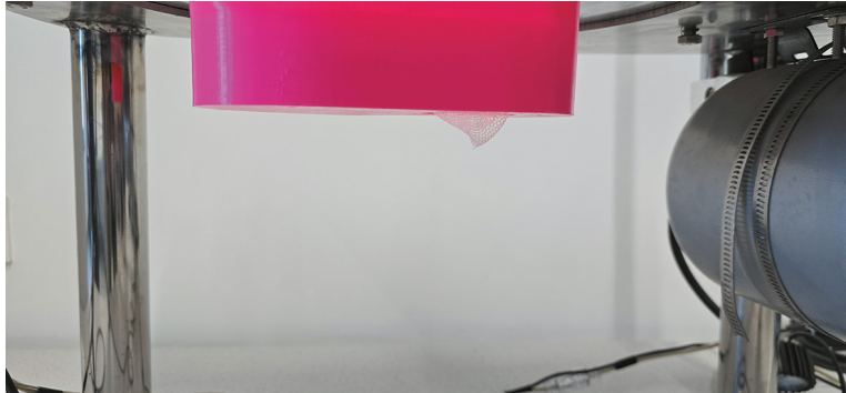
FIGURE 4 Representative image showing mesh displacement into the simulated defect under pressure. Displacement was defined as loss of overlap or protrusion through the defect, corresponding to early recurrence in the model.
