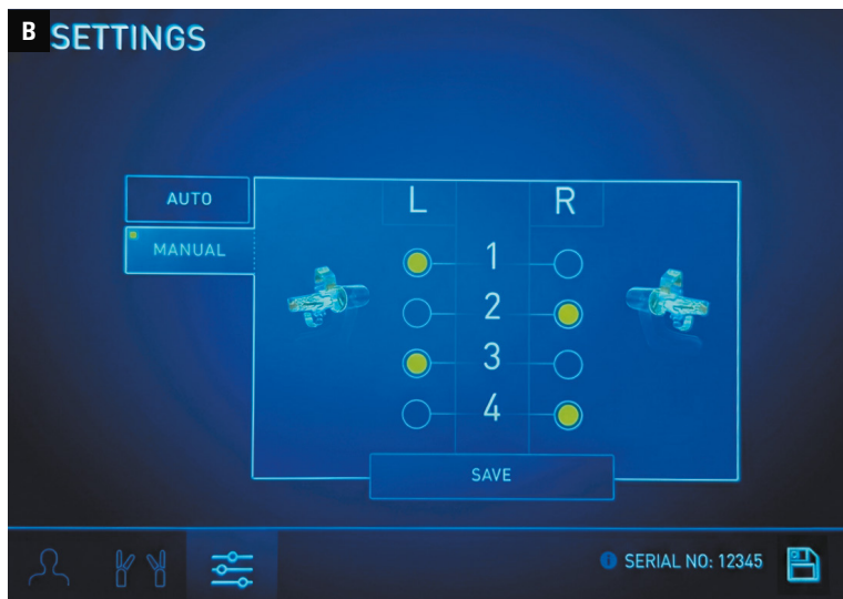
FIGURE 3 Manual hand assignment settings on the surgeon console touchpad; A – left-sided setup, with arms 1, 2, and 3 docked. Arm 2 is assigned to the left hand (L), and arm 1 to the right hand (R). Arm 4 (undocked) is also assigned to R to complete the circuit; B – right-sided setup, with arms 2, 3, and 4 docked. Arm 3 is assigned to L, and arm 4 to R. Arm 1 (undocked) is assigned to L.
